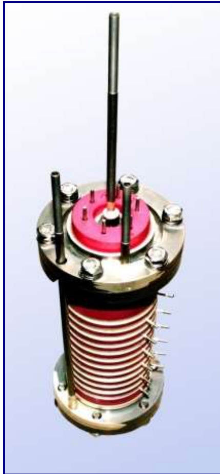
Metal ceramic camera for toxic gas and explosives analyzer
